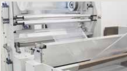
Film originating from "flat head" extruder
